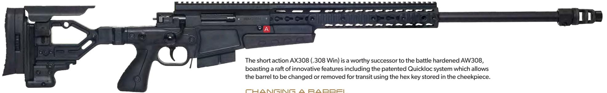
The short action AX308 (.308 Win) is a worthy successor to the battle hardened AW308, boasting a raft of innovative features including the patented Quickloc system which allows the barrel to be changed or removed for transit using the hex key stored in the cheekpiece.
